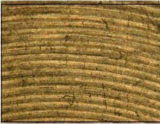
Fig.8 Microphotograph of machine surface with 50x magnification.
