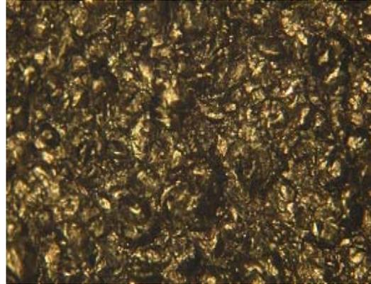
Fig.9 Microphotograph of peened surface with 50x magnification
