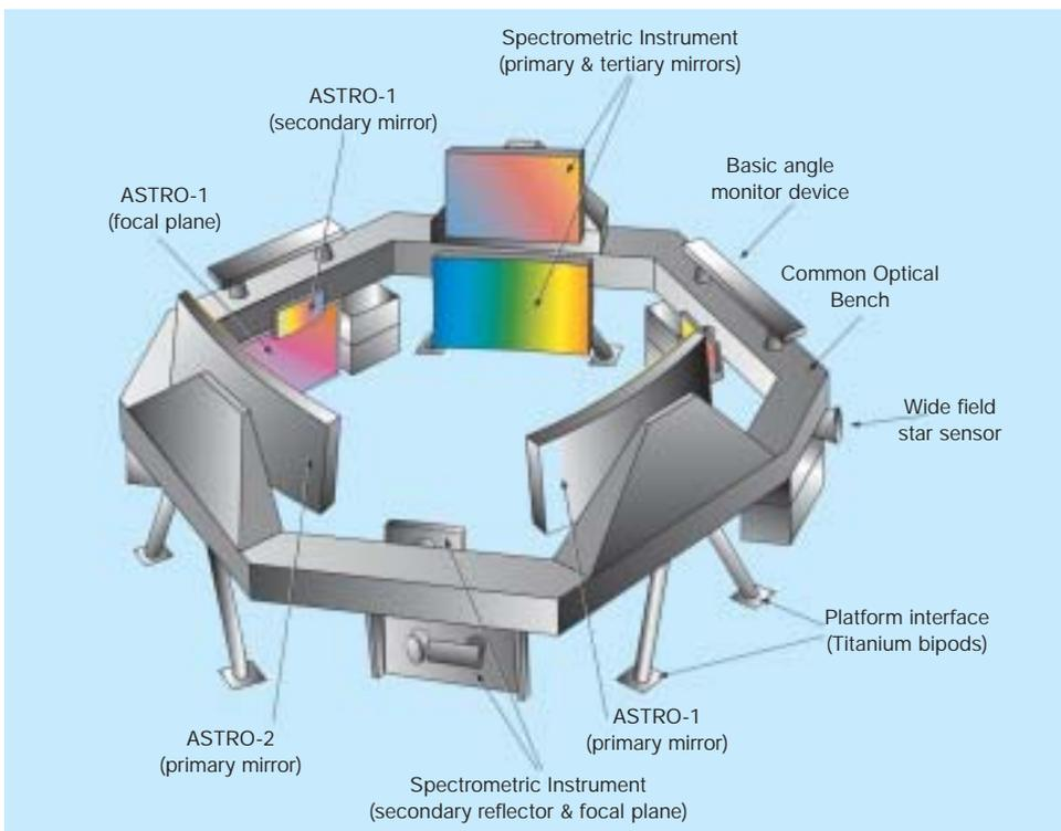
Figure 2. The GAIA three-mirror spectrometer
