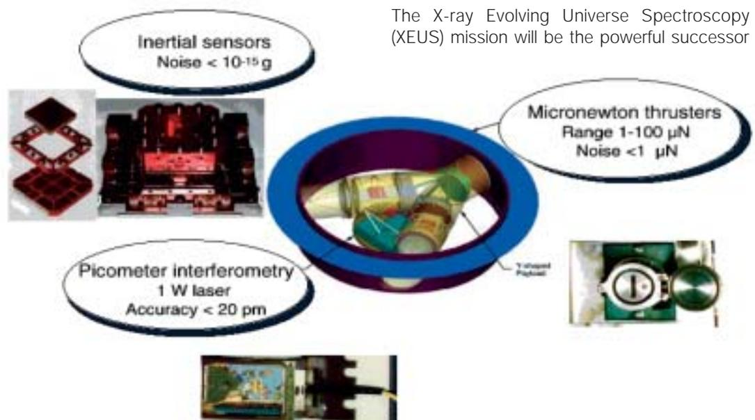
Figure 6. SMART-2 key technologies
