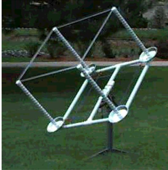
Our four antennas were positioned on the corners of a 1 m by 1 m square. A support structure made of PVC pipe (outer diameter = 4.25 cm) held the antennas in place. The antennas were connected electrically by coaxial cables which ran inside the pipes. The support structure was made of four PVC elbows, three PVC tees, six 45.3 cm lengths of PVC pipe, and two 95.5 cm lengths of pipe. When assembled, the pieces of pipe made a 1 m by 1 m square (center to center) with a central crosspiece.
