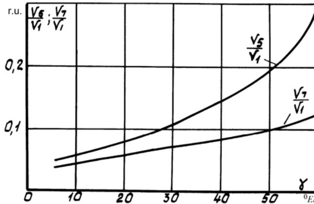
Fig. 5. The dependence of the harmonic 5-th and 7-th order voltage TSG from angle commutation RU
