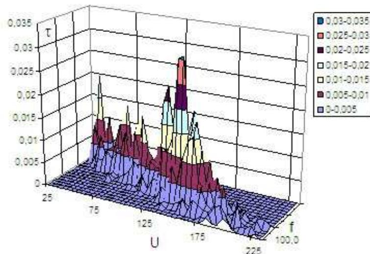
Fig. 2. Histogram of power modes AMF in the operation of the locomotive 2TE116
