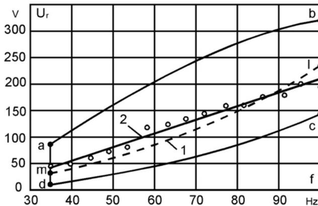
Fig. 1. Range of phase voltage  $U_p$  of the traction generator TC-501A (a, b, c, d) of the frequency  $f$ : 1 – of the frequency optimal law of supply for the AMF; 2 – average operational values  $U_p$
