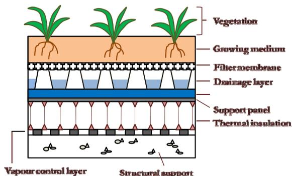
Figure 4. Structure of extensive green roof
