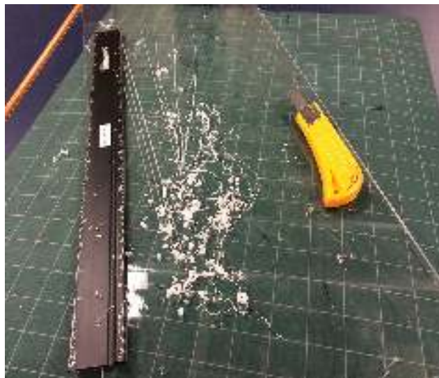
Fig. 1. Cut Plexi with Plexi cutter to make shavings to dissolve into paste.
