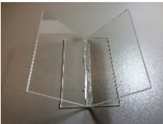
Fig. 5. One of the custom RBML Plexiglas cradles glued with quick and easy Plexi paste. The cradles survived travel to Germany and home using this paste.
