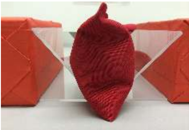
Fig. 4. After gluing out Plexi make sure to dry underweight in the fume hood.
