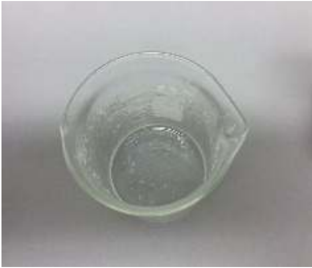
Fig. 3. Adding toluene to the paste will fully dissolve the mixture and it will become transparent and clear. Do not over mix!
