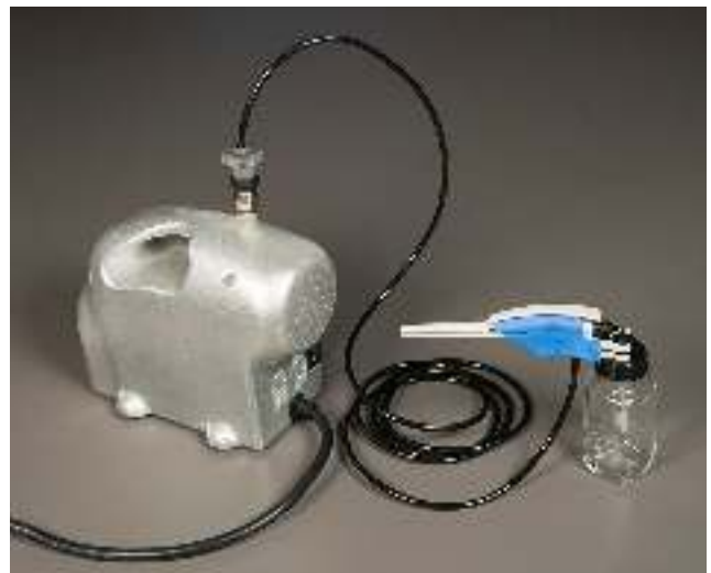
Fig. 2. Spraying the cellulose powder slurry onto Mylar using Testors® Multi-Purpose sprayer #8814 (This model was recently replaced with Testors® Basic Broad Stroke Airbrush System #A2207).
