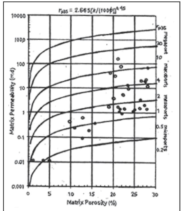
Fig. 4: Aguilera equation for pore throat aperture
