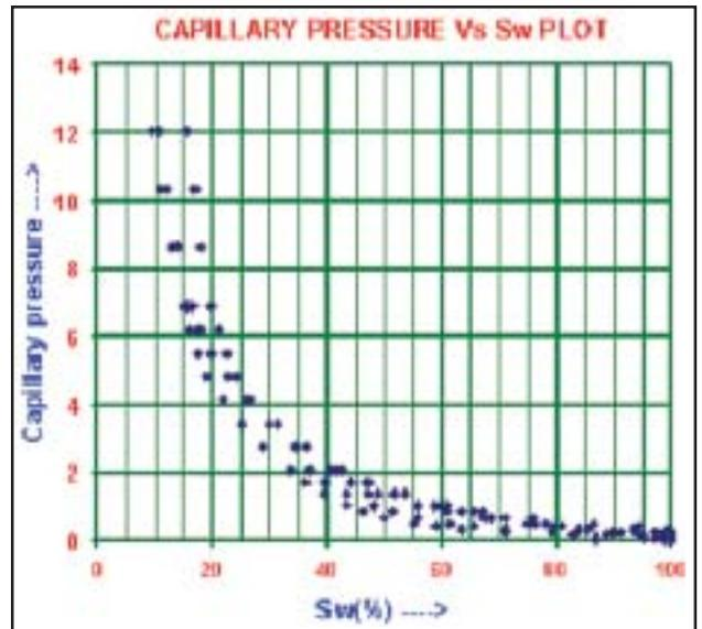
Fig. 5: Capillary pressure Vs Sw plot (core data).
