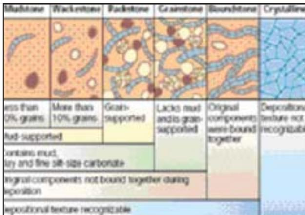
Fig. 1: Dunham classification of carbonate rock.
